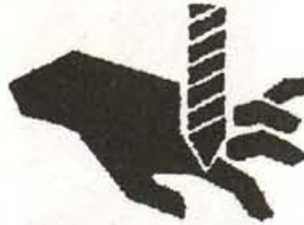
NEVER PLACE FINGERS NEAR CUTTING AREA OR MACHINE ARBOR
