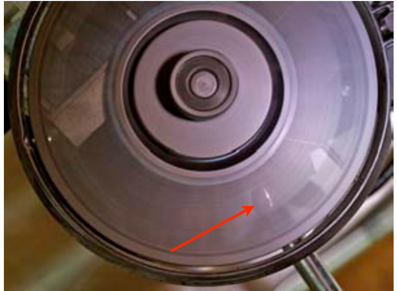
Here are close-ups of the slotted wheel in action. Note how you can see the very point of contact between the curved bevel and the abrasive.
