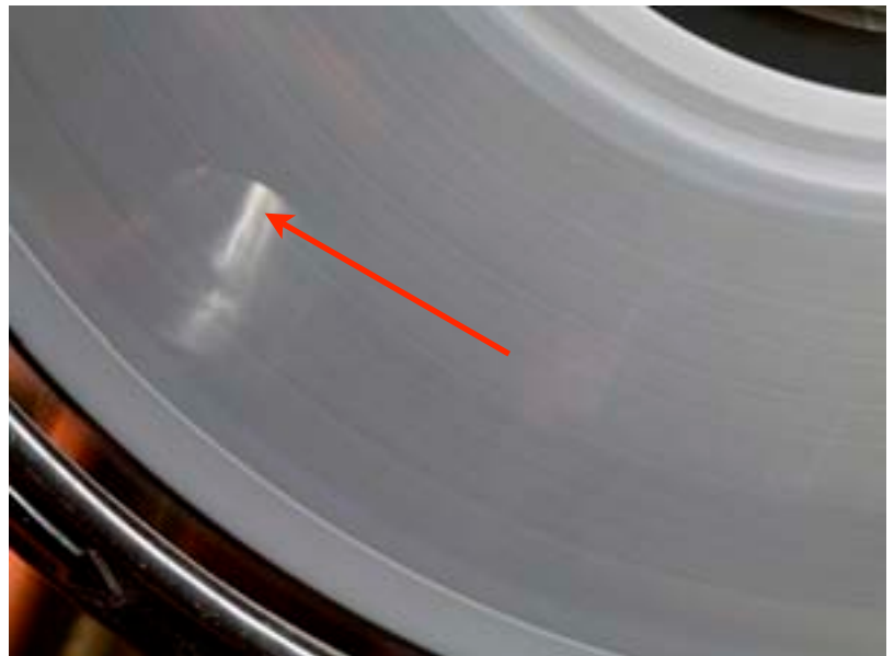
Here are close-ups of the slotted wheel in action. Note how you can see the very point of contact between the curved bevel and the abrasive.
