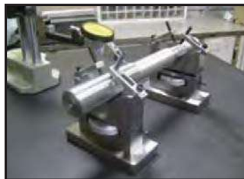
Adjustable Vee Block being used to check co-centricity of different diameters on a stepped rod
