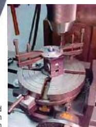
Parallel Clamps being used to hold a job for a precision drilling operation
