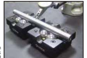
Ball Bearing Vee Blocks with non marring balls being used to check the roundness of a stepped rod
