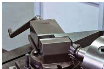
Milling machine vise being used to hold a job for milling operation.
